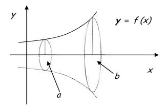
The diagram shows the graph of y = f(x) rotated 360° about the xaxis between x = a and x = b. The volume required is the region between the 2 dotted vertical lines and the 2 circles (which look like ellipses above due to perspective).
